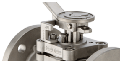
AZ plug valves are fitted with cast, rust proof position indicators. The position indicator is securely welded to the lever to prevent it from working loose.
