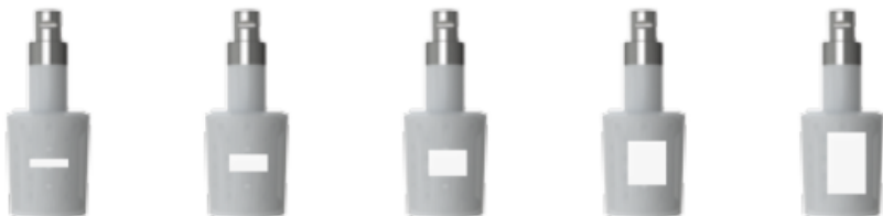
PTFE/PFA lined plug: linear control characteristics
